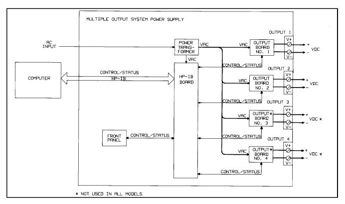
Figure 1-2. HP 6621A, 6624A and 6627A Multiple Output System Power Supplies, Block Diagram
